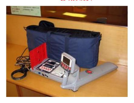
型号:接收机RD400 PXL/PDL2,发射机RD433HCTX-2
